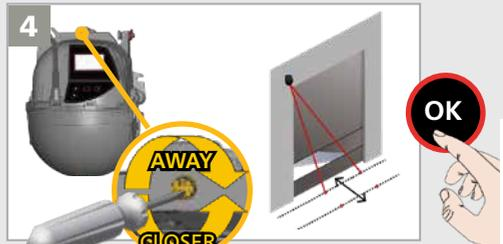
Position the curtain **closer to or further away** from the door by turning the screw at the top. Push OK to confirm.
