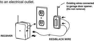
Note: Alternative wiring options are available, the receiver can be connected directly to the opener's motor. Please contact customer service for further information regarding alternative wiring options.
