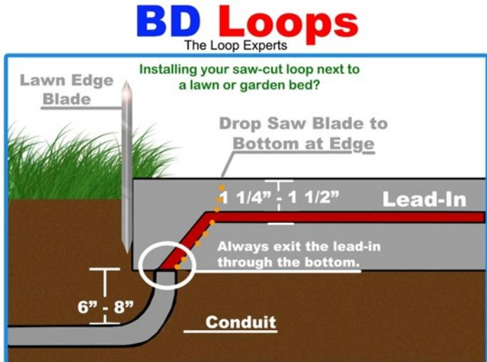
Lead-in should be run 6"-8" below the surface. Always run the lead-in through conduit
