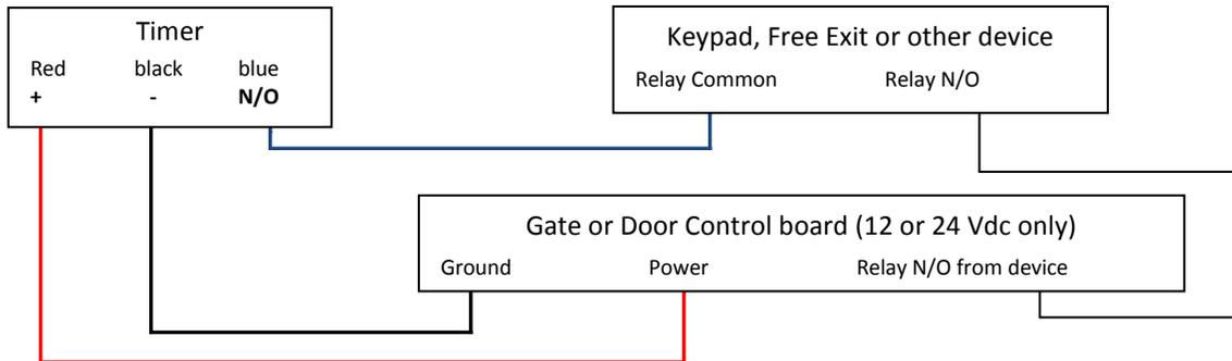
The illustration below shows how to wire the 7 day timer directly to a gate or door. The timer should be programmed with an ON time and OFF time corresponding to the time of the day the gate or door is to be held open. The close function must be part of the gate or door control board. The timer only holds the gate or door open overriding any automatic close function of the gate or door control board.
