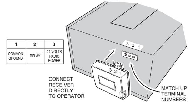
**STEP 1B SMDRG Installation (For non 24V Operator).** A Model TF524 step-down transformer must be used to power the receiver when connecting to an operator supplying anything other than 24V. Install the screws supplied into the brass terminals on the receiver. Connect the transformer wires to Terminals 1 & 3 (polarity not important). Connect receiver Terminals 1 & 2 to the two operator activation terminals (polarity not important).
