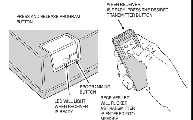
**STEP 6 Add additional transmitters.** Repeat Step 5 for each transmitter used with this receiver. Be sure to press the receiver's program button **each time a new transmitter or a different transmitter button on a multi-button transmitter is pressed.** If the LED doesn't come on when the receiver's program button is pressed, the receiver's memory is full (40 transmitters total). Use the erase function (Info 1) to remove **ALL** previously learned transmitters from the receiver's memory.
