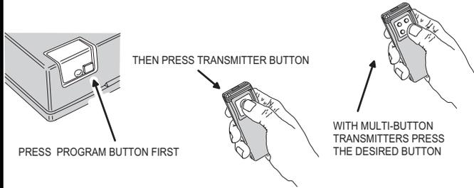
**STEP 7 Review memory.** Press and hold the receiver's program button until the LED begins to flash (about 3 seconds) and then release the button. Count the number of flashes. The number of flashes equals the number of transmitters programmed into the receiver.
