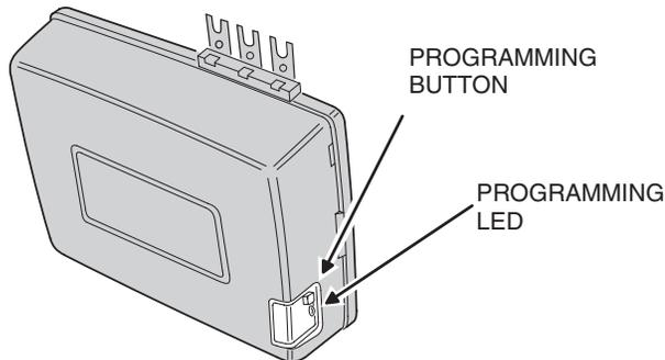
**STEP 5 Program receiver.** Momentarily press the receiver's program button. The red programming LED will light if there's room in the receiver's memory for another transmitter (40 maximum per receiver). The LED stays on for about 5 seconds. **A transmitter must be entered while the LED is on.** Press the desired transmitter button. The LED will flicker indicating that the receiver has accepted the transmitter.
