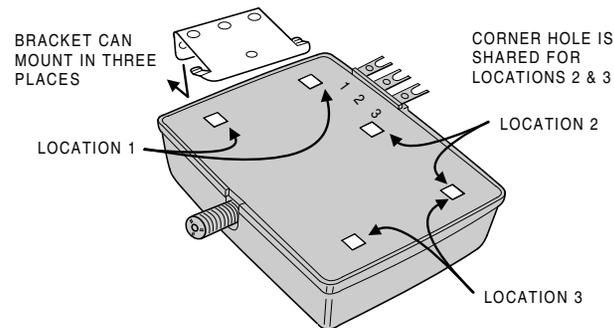
**STEP 3 Installing the antenna.** Attach the local antenna by screwing it onto the "F" connector.
