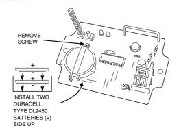
**STEP 9** *Program Transmitter.* Refer to receiver programming instructions to set the receiver into the program mode. Press the "test" button to program the unit identification code into the receiver. Facility/ID code is located on the inside of the unit, near the terminal block.
