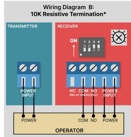
\*If you need a normally open relay, but without a 10K resistor then set Dipswitch 4 to OFF. This is a non-monitored method.
