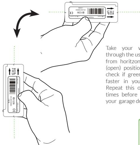
Take your wireless sensor and through the use of your hand, change from horizontal (close) to vertical (open) position (or viceversa) and check if green STATUS light blinks faster in your Gogogate2 device. Repeat this operation a few more times before placing the sensor in your garage door.
