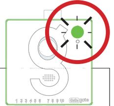
**NB:** Check if green STATUS light blinks faster in your Gogogate2 device. If so, your wireless sensor is transmitting signal properly to Gogogate 2 device.
