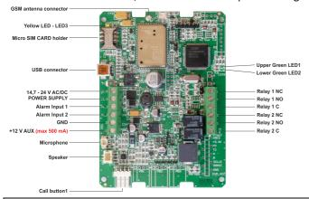
Do not use the +12V AUX power output for electric lock driving! You can use it to power external sensors only (500mA max)! Use separate power source for door electric lock!
