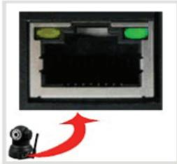
After cables are connected, the indicators on the Ethernet jack should be lighted as the right top figure: the yellow one flashes and the green one keeps on. If it's not the case, please check:
