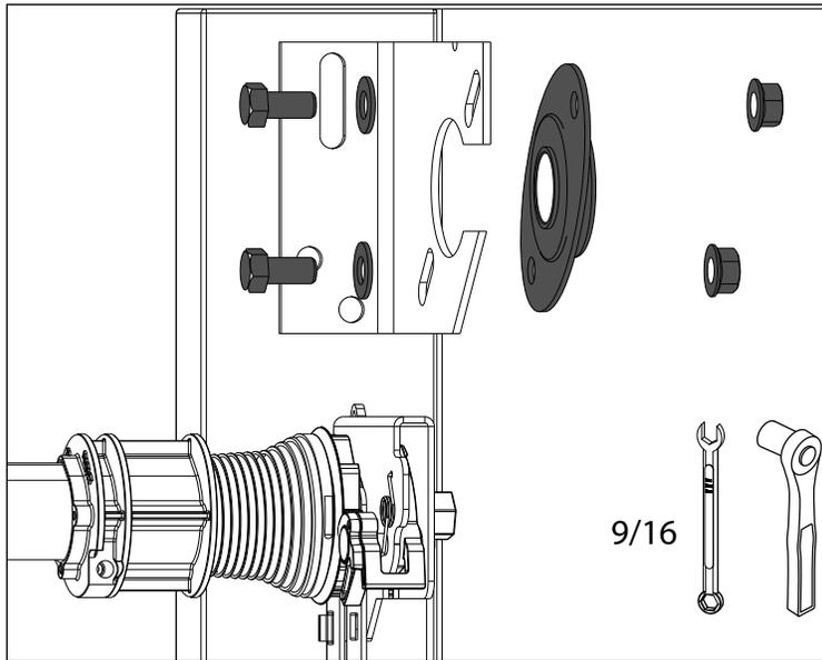
7. Loosely install oval bearing plates with bolts, washers and nuts provided on the right side of each bracket.
