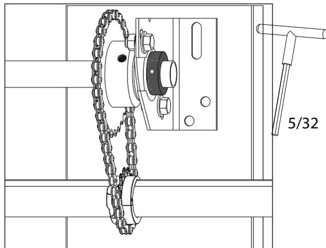
12. Ensure 28T sprocket is seated against inside bearing.
