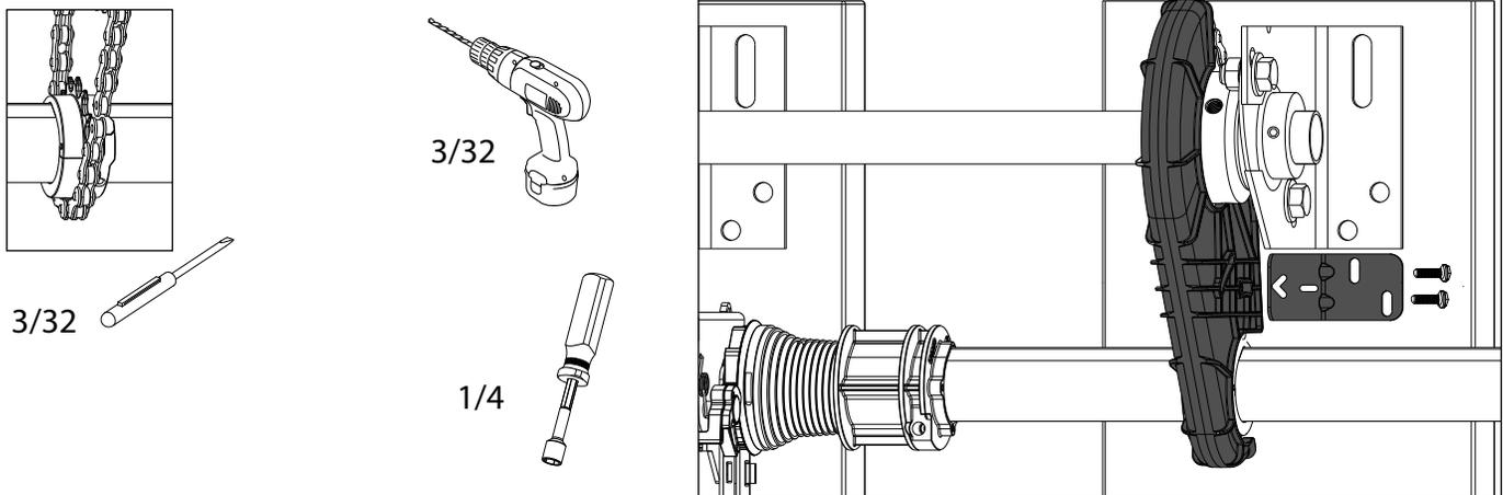
17. Install supplied bracket screws into cover.
