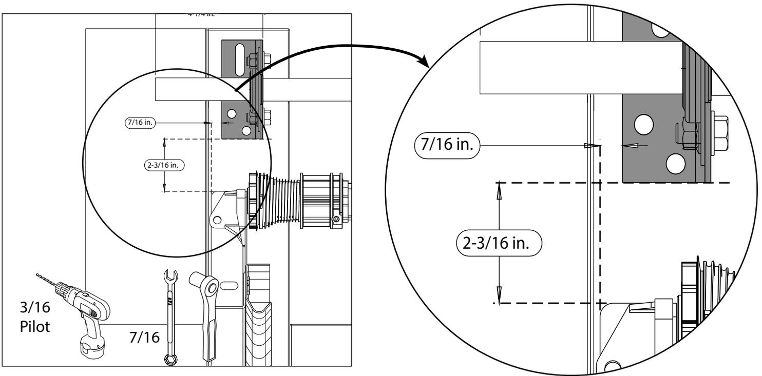
2. Measure up from the TorqueMaster® mounting bracket 2-3/16 in. and mark a horizontal line.
