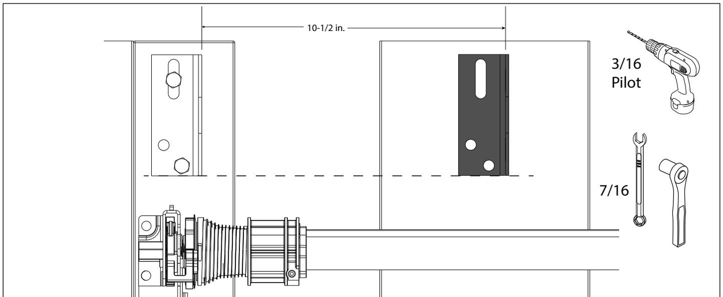
5. Measure in 10-1/2 in. and mark mounting surface for position of inner bracket.
