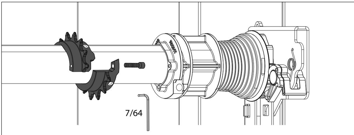
11. Install 2-piece sprocket onto TorqueMaster® shaft and assemble using a 7/64 in. allen wrench.
