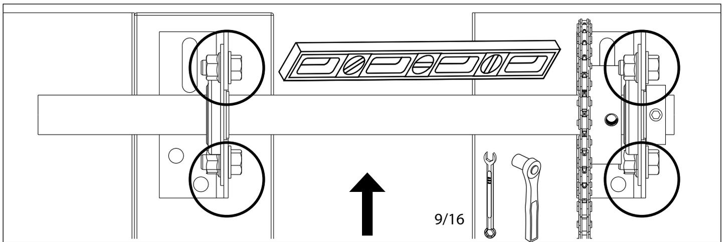
15. Align sprockets and push up on drive shaft to tighten chain, ensure shaft is level and tighten bearing bolts and nuts.
