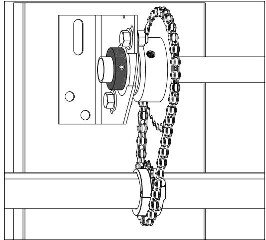
12. Ensure 28T sprocket is seated against inside bearing.
