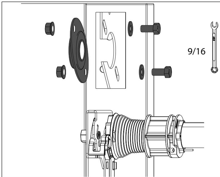
7. Loosely install bearing plates with bolts, washers and nuts provided on the left side of each bracket
