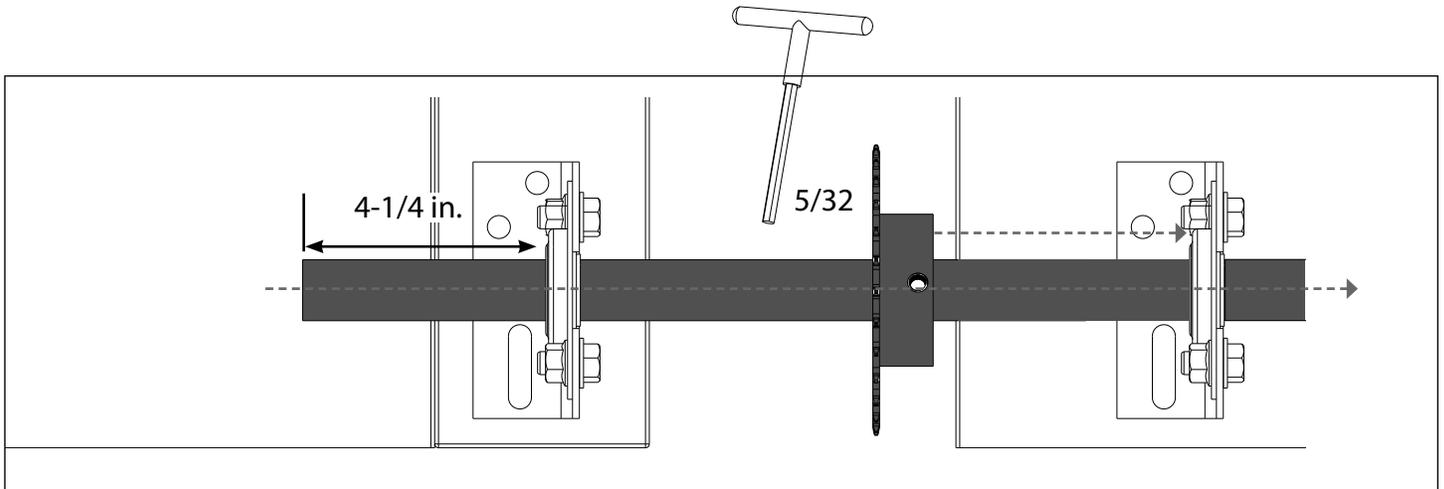
8. Slide 28T sprocket onto drive shaft and slide into bearings.
