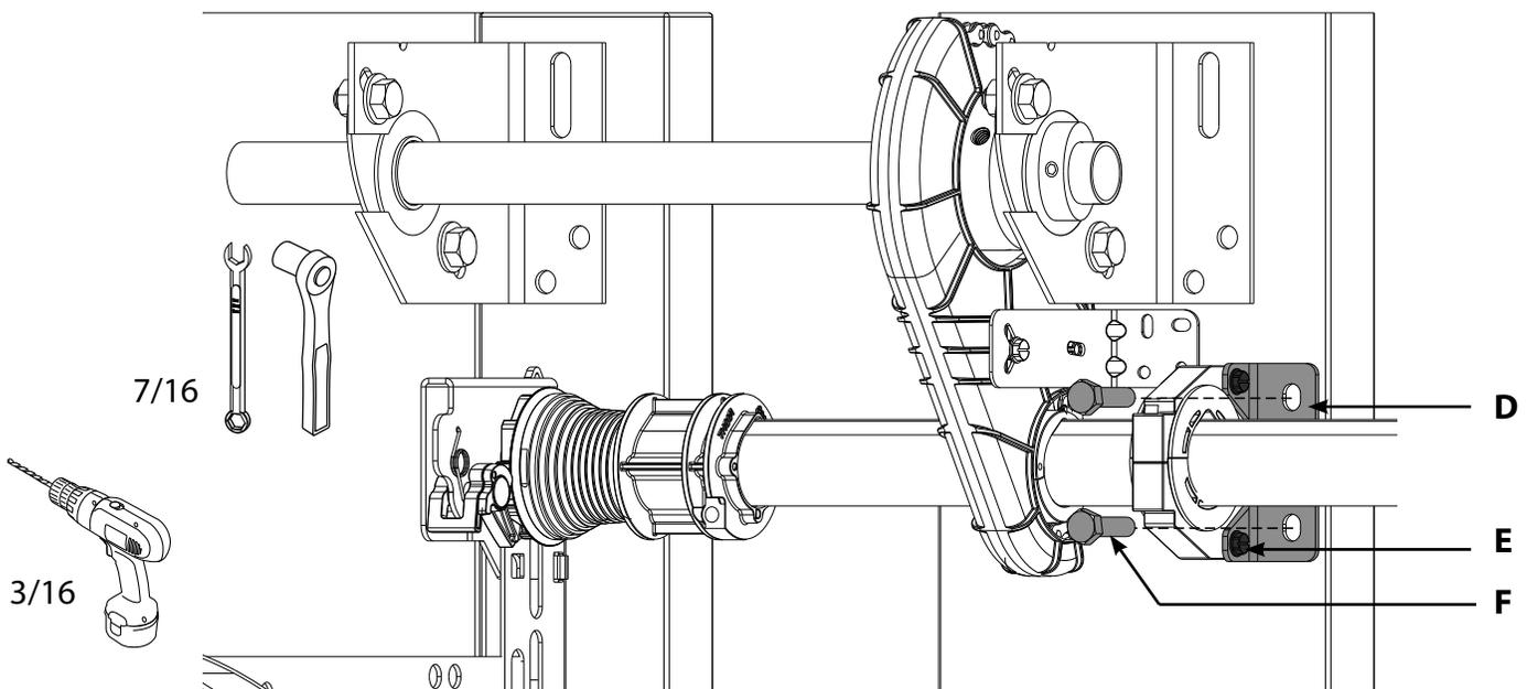
5. Install opener onto drive shaft per openers installation manual instructions.
