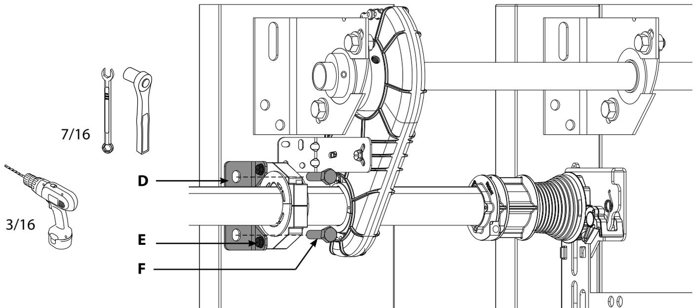
23. Install opener onto drive shaft per openers installation manual instructions.
