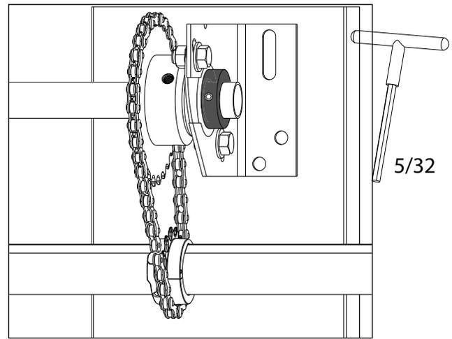
12. Ensure 28T sprocket is seated against inside bearing.
