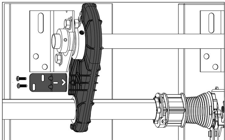
17. Install supplied bracket screws into cover.
