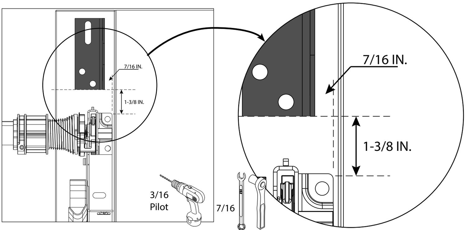
2. Measure up from the TorqueMaster® mounting bracket 1-3/8 in. and mark a level horizontal line.
