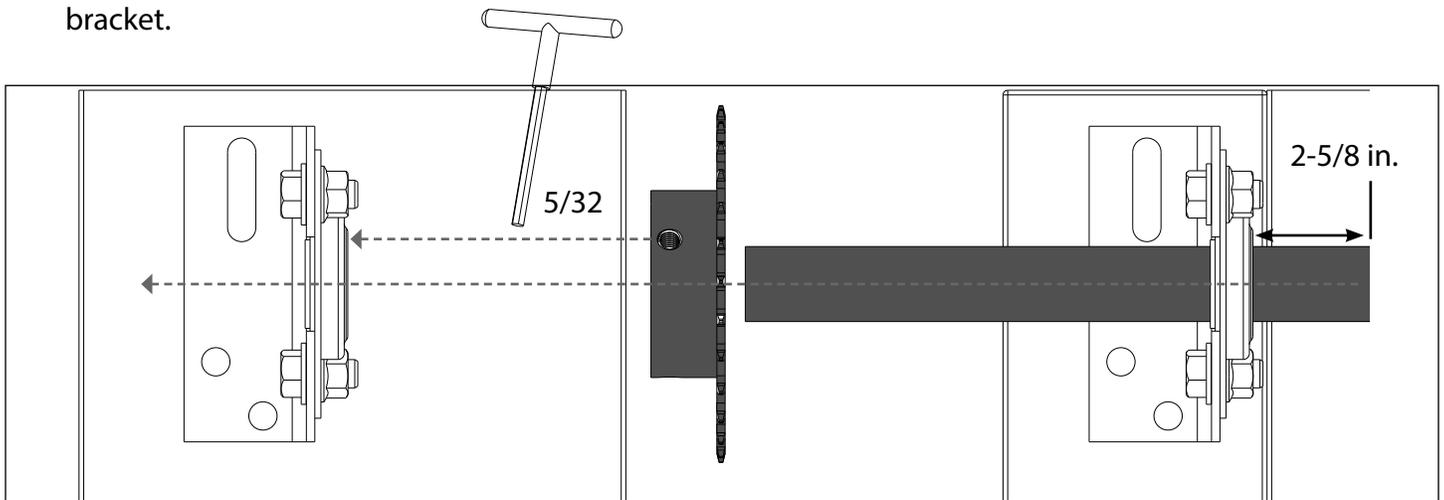
8. Slide 28T sprocket onto drive shaft and slide into bearings.
