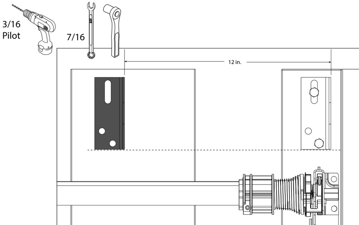
5. Measure in 12 in. and mark mounting surface for position of inner bracket.
