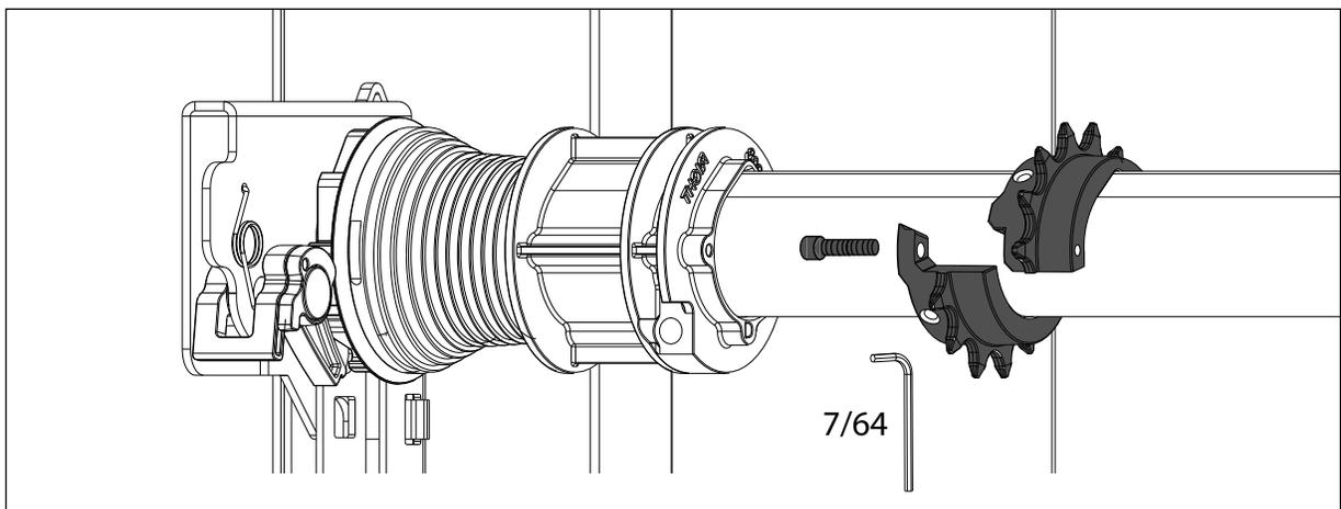
11. Install 2-piece drive sprocket onto TorqueMaster® shaft and assemble using a 7/64 in. allen wrench.
