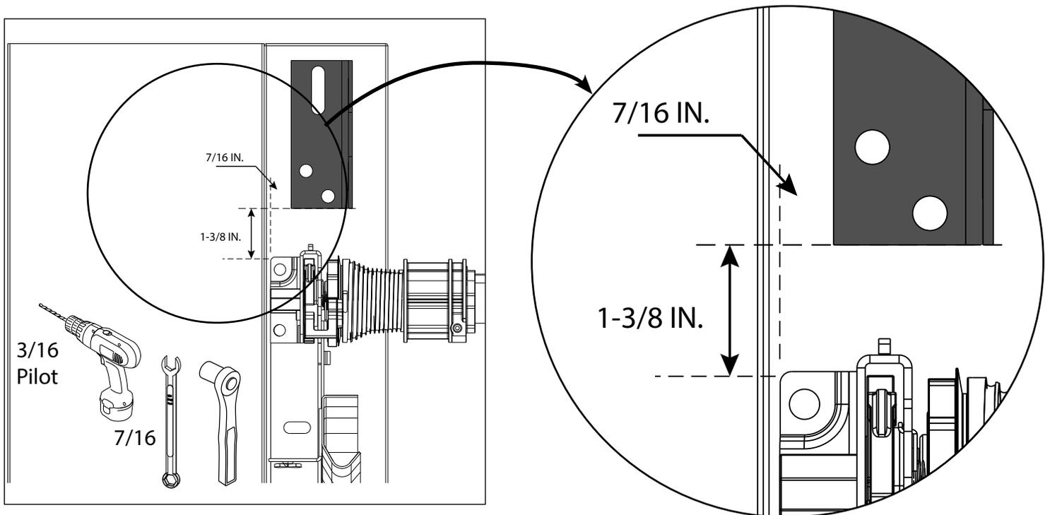
2. Measure up from the TorqueMaster® mounting bracket 1-3/8 in. and mark a horizontal line.
