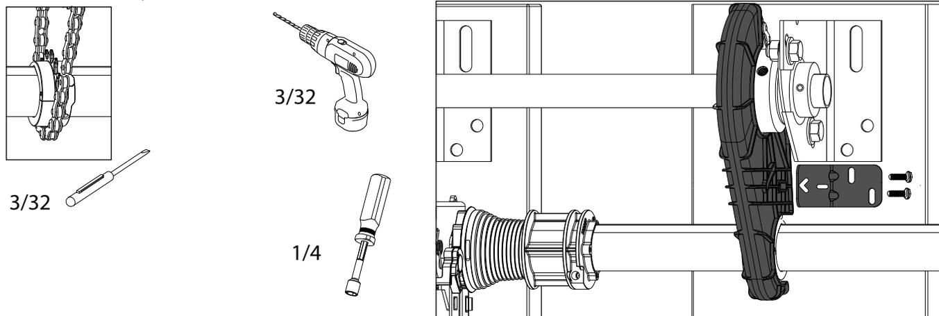
17. Install supplied bracket screws into cover.
