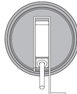
Image 4: Aligning the Emitter/Receiver with the Reflector
