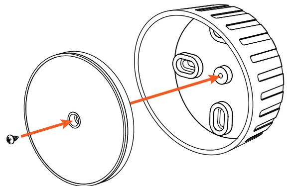
**Image 2: Reflector with Hood & Center Screw**
