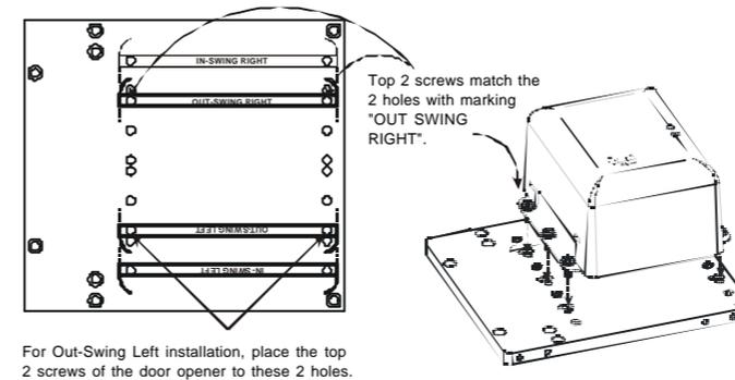
For Out-Swing Left installation, place the top 2 screws of the door opener to these 2 holes.
