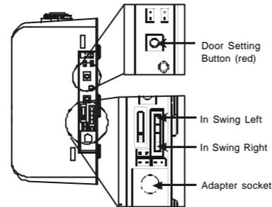
Step 1) Press and hold the door setting button. (red)
