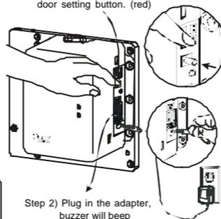
Step 2) Plug in the adapter, buzzer will beep rapidly.
