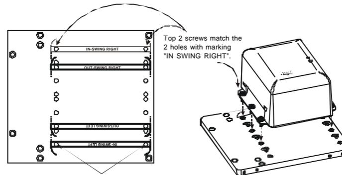
For In-Swing Left installation, place the top 2 screws of the door opener to these 2 holes.
