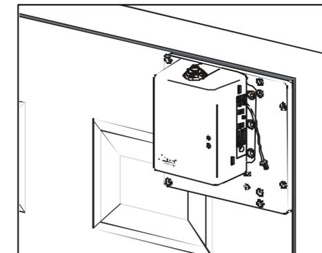
5.3 Secure the mounting plate with 4 screws onto the door.
