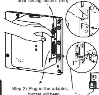
Step 2) Plug in the adapter, buzzer will beep rapidly.
