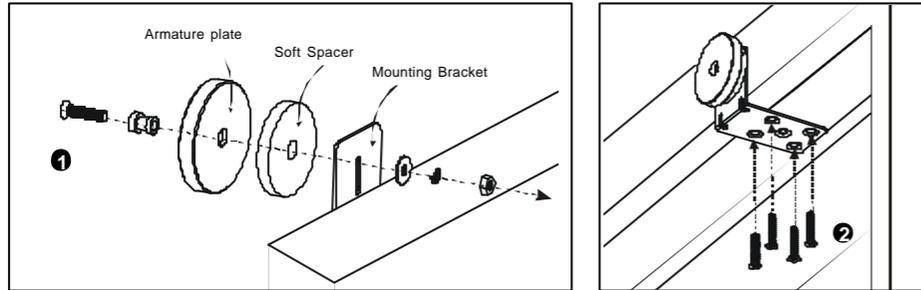
8.2 Secure the armature plate mounting bracket and spacer on the upper corner of the top door jamb with the armature screw, eyelet and a washer.
