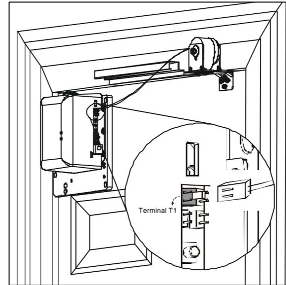
If the wire is too long, you may use a cable tie or tape to secure the wire on the door.
