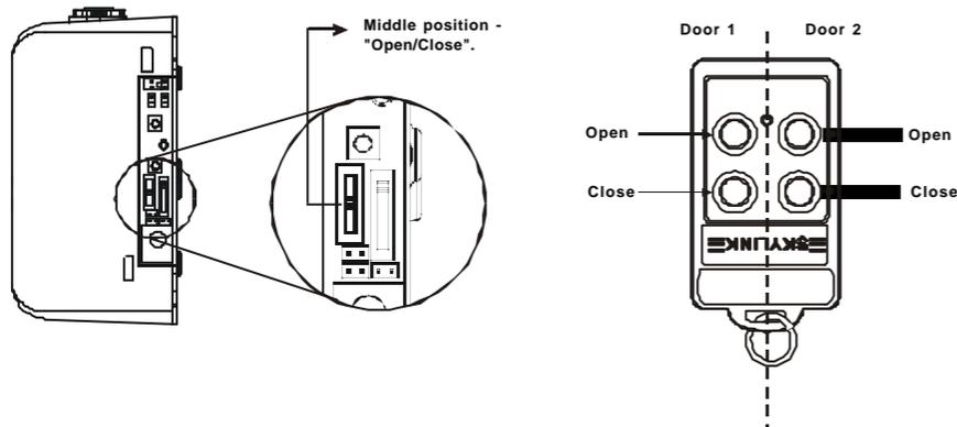
A 4-button remote control allows you to operate 2 different door openers. If you would like to operate Door 1, both the open and close buttons of door 1 must be programmed to the door opener. Follow the instructions for "Learning Remote Controls" on page 28. If you would like to operate another door opener using the same remote, learn the other 2 buttons to the other door opener.
