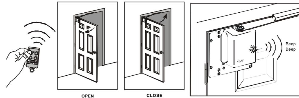
If you would like to stop the door when it is either opening or closing, you can press the remote button 1 again, it will stop the operator therefore stopping the door from opening / closing.
