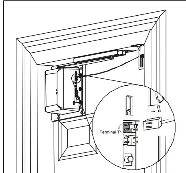
If the wire is too long, you may use a cable tie or tape to secure the wire on the door.
