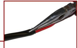
**This Splice Kit is not designed for wire thinner than 16 AWG.**
