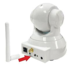
2. Plug network cable into camera and into your router. (You can unplug this once WiFi is setup).
