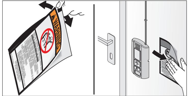
1. Attach the warning labels in an visible area of the garage (for example near the wall station).
