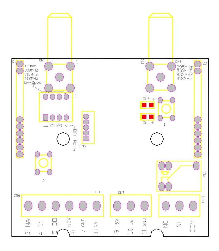
The RCS-UR Receiver is a configurable Receiver Processor that can work with 6 different frequencies: 295MHz, 318MHz, 418MHz, 433MHz, 310MHz, and 300MHz.
