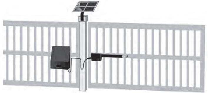
When deciding where to mount the control box remember the actuator cable is 8 feet in length. If possible, mount the control box in a location that will allow the cable to be neatly routed. If it must be longer than the 8 feet, see Splicing Actuator Cable Step. Also avoid choosing a mounting location that is near sprinklers.
