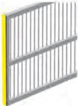
**Zone A** - Leading edge of gate where it meets a 2nd gate, stop post or passes a column or post corner. - recommended monitored entrapment protection type is B2 contact sensor or equivalent.
