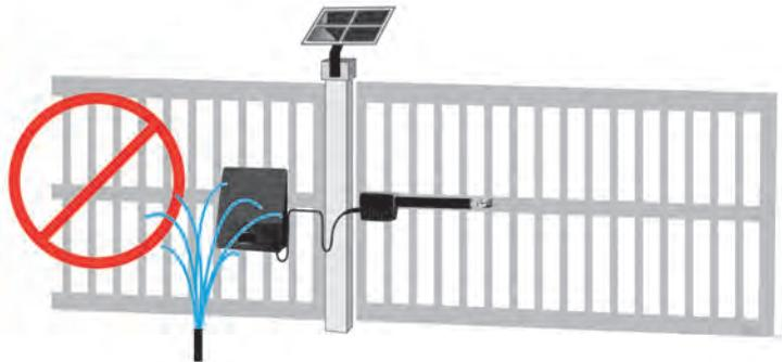
We have provided knockouts for conduit fittings in the control box bottom right corner. We highly recommend using conduit for all accessory wiring entering the control box. Determine which knockouts are to be used and punch out at this time.
