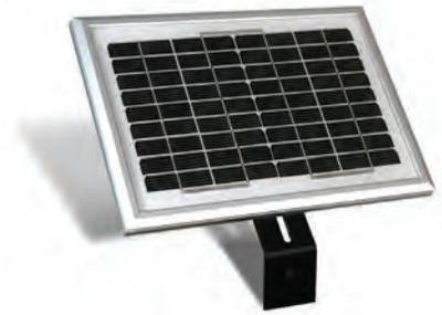
The solar option allows you to install the gate operator in remote areas or in applications where you prefer to be solar charged. Solar charging provides isolation from lightning that might damage the unit via the AC power needed for the transformer. The use of solar friendly accessories will help prevent premature battery failure.
