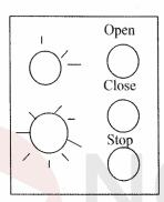
Open, Close & Stop Transmitter to Control 27 Doors. Match dipswitches 1 thru 5 on both transmitter and receiver. Set the 6th, 7th, & 8th dipswitch in open/close/stop receiver accordingly.
