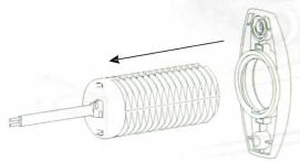
2. Mount clip to guide or surface using screws and spring.
