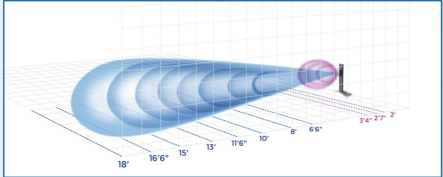
Microwave detection patterns (blue above) are adjustable from 7 to 18 feet. The Ultrasonic Sensor is for close range detection (purple). The OVS-01GT Vehicle Virtual Loop also features 5 sensitivity settings.
