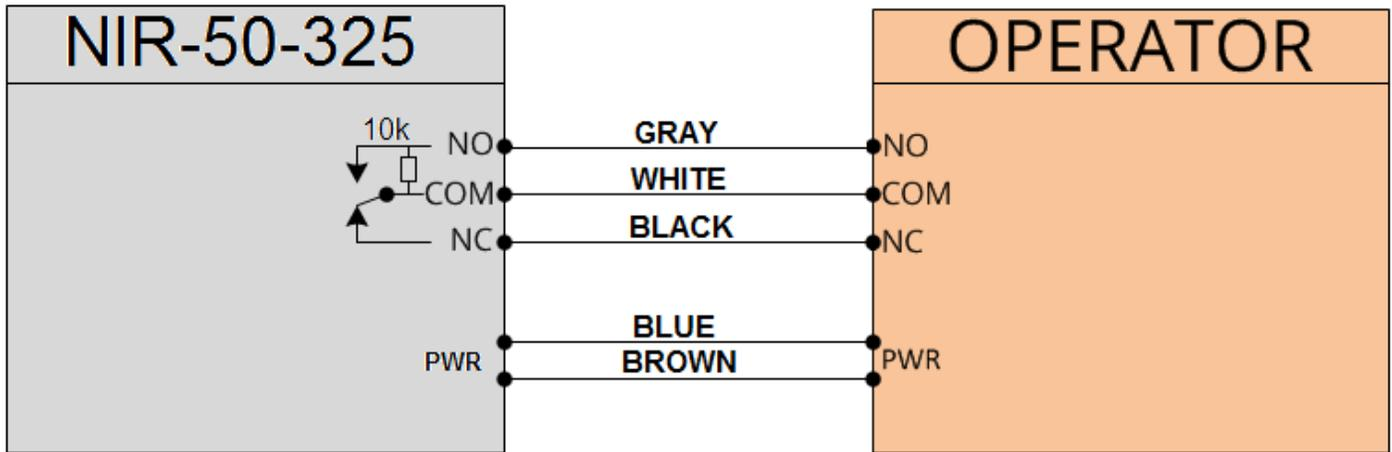
NOTE: The relay contacts on the board and the references to them in these instructions are shown in the energized state, aligned with reflector and no obstruction
