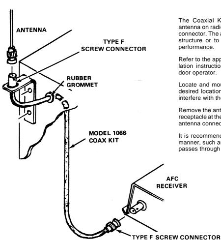
The Coaxial Kit permits the remote location of the antenna on radio receivers equipped with a type F screw connector. The antenna can be moved away from a metal structure or to an outside location for better receiver performance.
