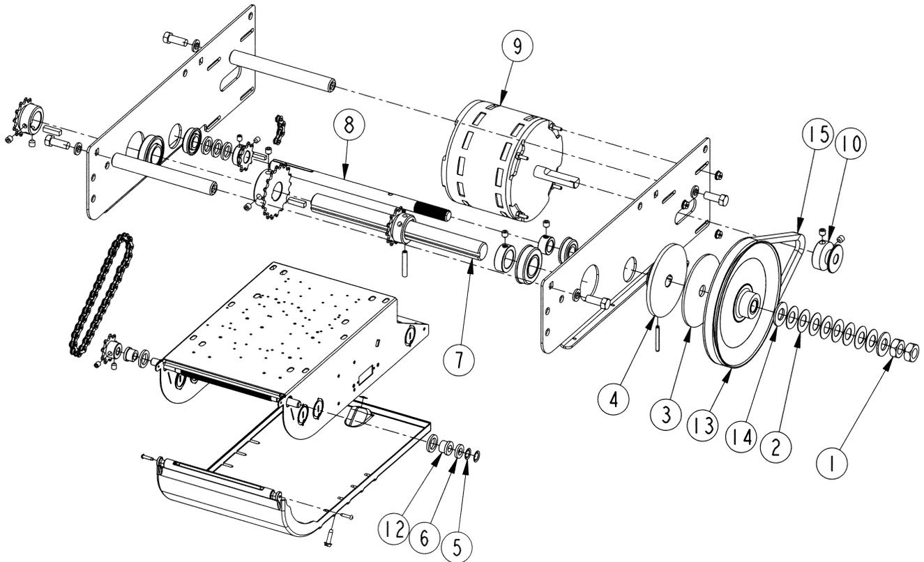
Figure 33 - OMT Mechanical Exploded View
