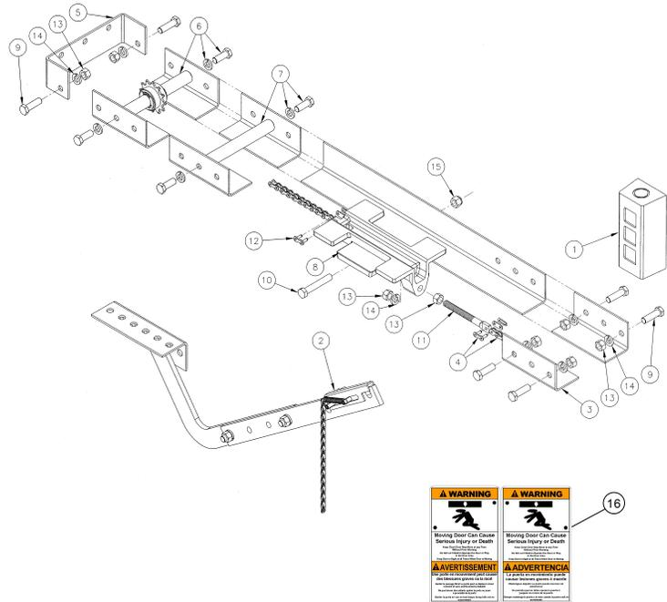
Figure 2 - Standard Trolley Hardware
