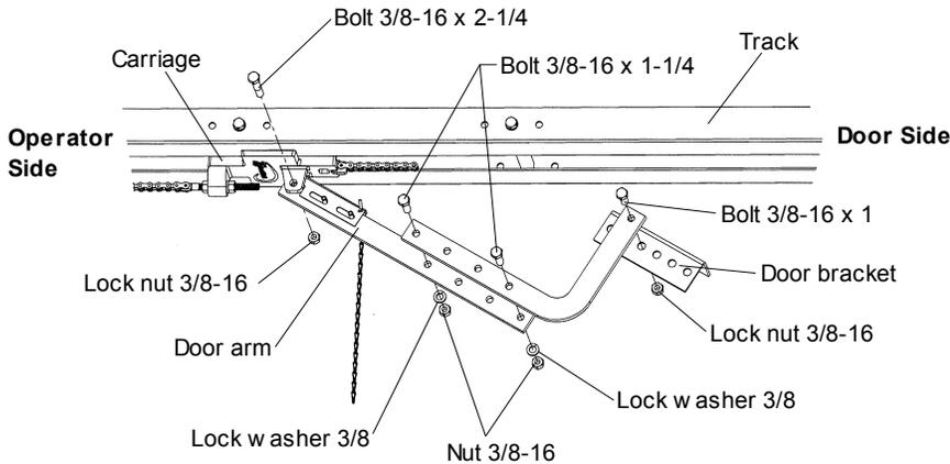
Attach door arm to door using appropriate fasteners. Mount door bracket to the center of the door.
