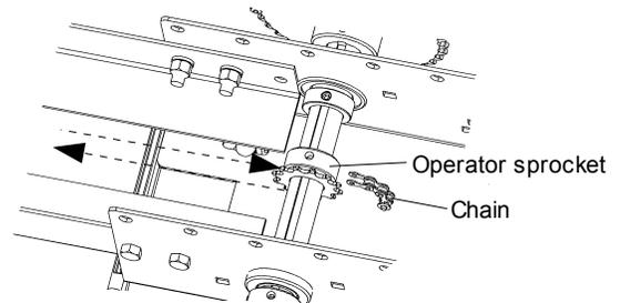
D) Attach chain to back of carriage.
