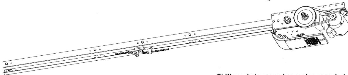
C) Wrap chain around operator sprocket.
