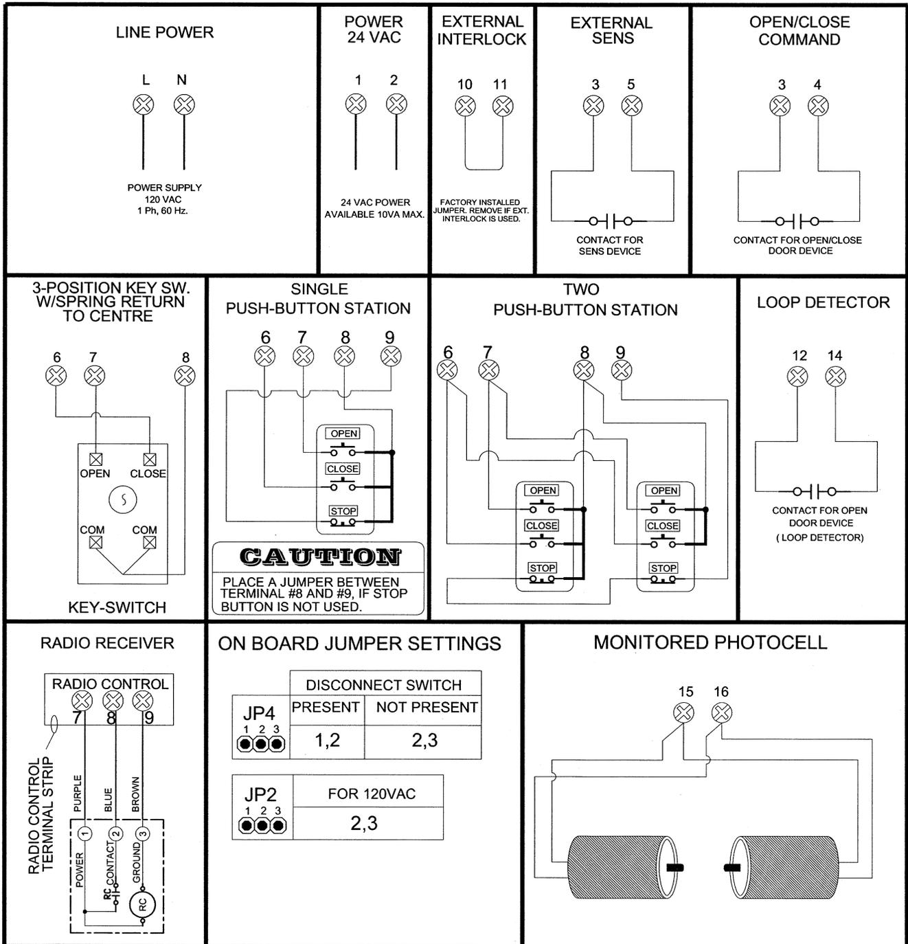
Figure 32 - External Wiring
