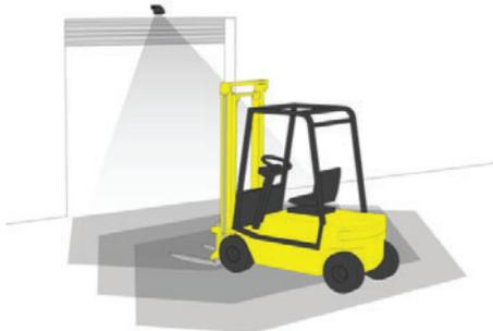
**Vehicle approaches:** Vehicle-detection relay is activated. Door opens.
