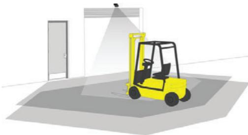
**Vehicle approaches:** Vehicle-detection relay is activated. Door opens. Person-detection relay is not activated. Entrance for people remains locked.
