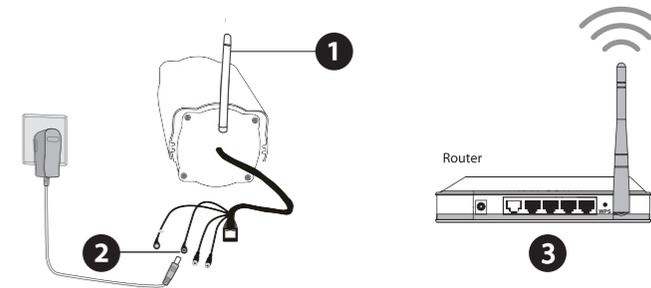
1. Turn on your iSmartgate IP Camera using the provided power supply. (do NOT use the Ethernet - RJ45 cable).
