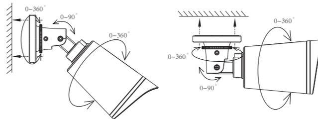
Place the camera on your preferred location and use the supplied mounting screws to fix the camera securely.
