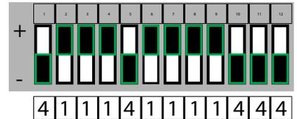
**STEP 1: Each shaded box below represents a DIP switch position.** In these boxes, write in the number 1, 2 or 4 as it corresponds to the UP, MIDDLE or DOWN switch position you see on the remote, opener head or receiver.
