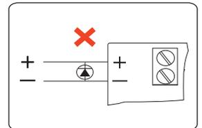
Remove any diode and varistor to prevent the door from delayed opening.
