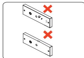
Make sure the faces of the magnetic lock and the armature plate are clean, intact and no rust.
