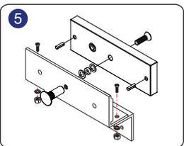
Fasten armature plate to Z bracket. Add plastic washers between bracket and armature plate.
