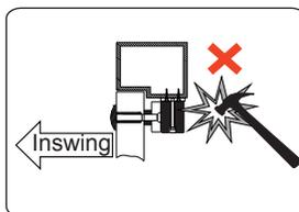
The magnetic lock and wires must not be exposed. Install LZ bracket for inswing doors.
