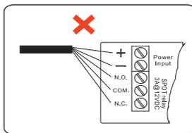
Do not apply power wires and signal wires in the same cable or conduit.
