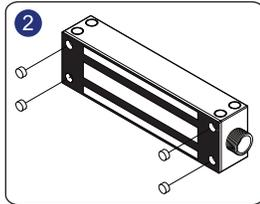
Insert caps into screw holes in maglock.
