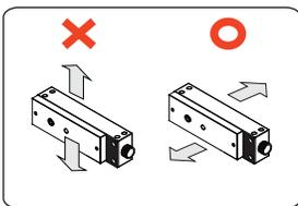
The magnetic lock must face-to-face align with the armature plate or the holding force will decrease by 25%.
