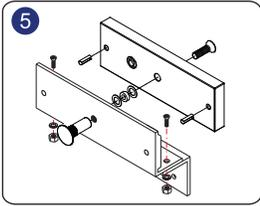
Fasten armature plate to Z bracket. The rubber washer must be placed between the armature plate and the bracket.
