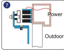
After the armature plate and the magnetic lock stick to each other, adjust the Z bracket to fit the door frame.
