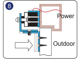
Adjust and fasten the Z bracket. Close the door and test the holding force. Adjust the gap between the armature plate and the magnetic lock by adding or removing the washers or by tightening the armature plate.
