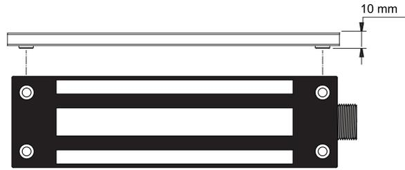
Thickness of 10 mm with enhanced sturdiness to secure the magnetic lock
