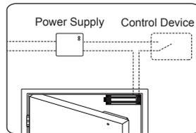
The magnetic lock is fail-safe. It requires a UPS to supply power to keep the door locked during power failure.
