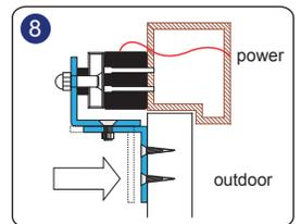
Adjust and fasten upper part of Z bracket. Close door and test holding force. Adjust the gap between armature plate and maglocks by adding or removing washers or tightening the armature plate.
