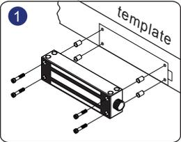
Drill holes as shown on template and fit blind nuts into holds. Fit maglocks with hex-socket head screws.
