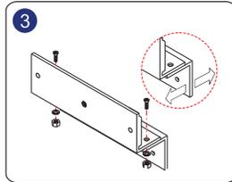
Assemble Z bracket. Note that the bracket is movable.
