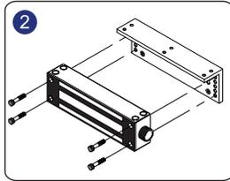
Fasten the magnetic lock to the L bracket with hex-socket head screws.
