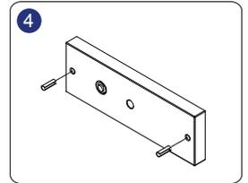
Insert guide pins into armature plate (to fix it).
