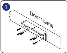
Install the L bracket to the mounting position on the door frame. Make sure the door can be freely opened.
