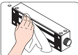
Regularly wipe the surface of the magnetic lock with anti-rust oil.
