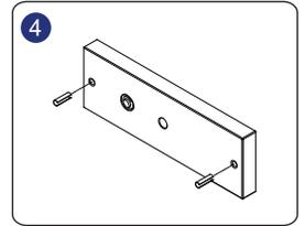
Insert the guide pins into the armature plate.
