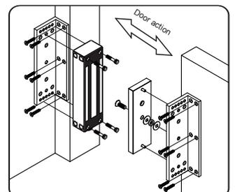
Fit L-GL1200FS-IOTB bracket on sliding doors and frames.
