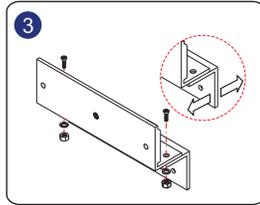
Assemble the Z bracket. Note that the bracket is movable.
