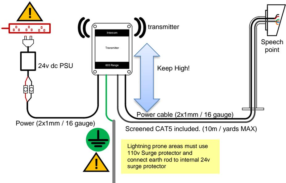
**Tip:** For shorter distances, some installs may mount transmitter on pedestal for convenience. Range test first! For high security applications, it is recommended to locate the transmitter INSIDE the property perimeter.
