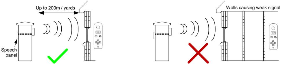
**Tip:** For longer range installations, locate the handset close to the front of the property, near a window if possible. Concrete walls can reduce the open-air range of 400 metres/yards by 30-50% per wall.
