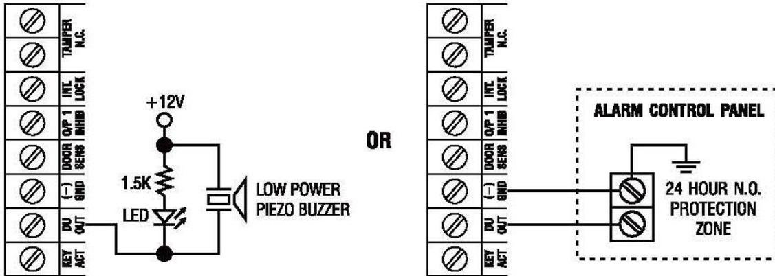
The Duress Output will switch to (-) ground when duress code is entered. You may use it to turn ON an LED lamp and /or a small buzzer to notify a guard; or connect it to a 24 hour Normally Open protection zone of an alarm system.
