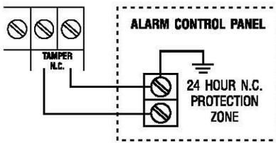
The tamper switch is Normally Closed while the keypad is secured on gang box. It is open when the keypad is removed from the gang box. To prevent sabotage, connect these terminals in series with a 24 hour N.C. protection zone of an alarm system if required.
