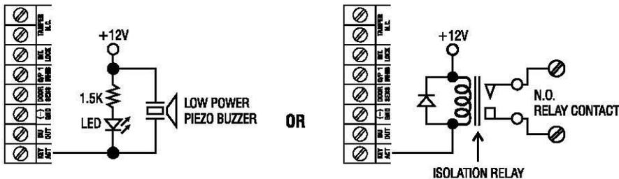
The Key Active Output will switch to (-) ground for 10 seconds whenever a key is touched. You may use it to turn ON an LED lamp and /or a small buzzer to notify a guard; or to energize a relay to switch ON lights or trigger an CCTV Camera to start recording.
