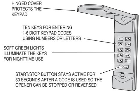
START/STOP BUTTON STAYS ACTIVE FOR 30 SECONDS AFTER A CODE IS USED SO THE OPENER CAN BE STOPPED OR REVERSED
