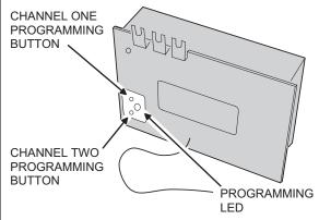
**STEP 5** Program receiver. Momentarily press the receiver's program button (channel one or two). The red programming LED will light if there's room in the receiver's memory for another transmitter (10 maximum per receiver). The LED stays on for about 5 seconds. A transmitter must be entered while the LED is on. Press the desired transmitter button. The LED will flicker indicating that the receiver has accepted the transmitter.
