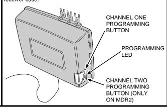
**STEP 4B** MDRM/MDRM2 Program button and LED Location. Locate the program button and LED on the back of the receiver case.
