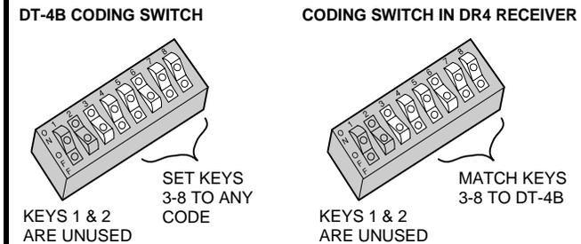
**STEP 3 Test the equipment.** Connect the receiver(s) to the operators as described in the receiver's installation instructions. **Be sure the door/gate area is clear.** Activate the transmitter and verify that the receiver triggers the operator. Check that the correct button on the DT-4B activates the desired operator.
