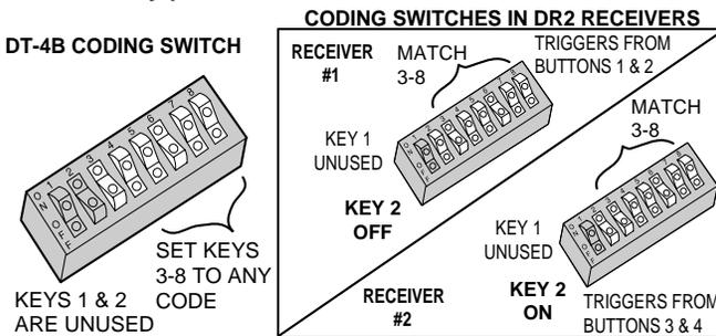
**STEP 2C Coding for a four-channel receiver.** Pick any combination of OFF/ON codes and set them on switch keys 3-8 in the transmitter. Match the same code on switch keys 3-8 in each receiver. **Transmitter and receiver switch keys 1 & 2 are unused and can be in any position.**
