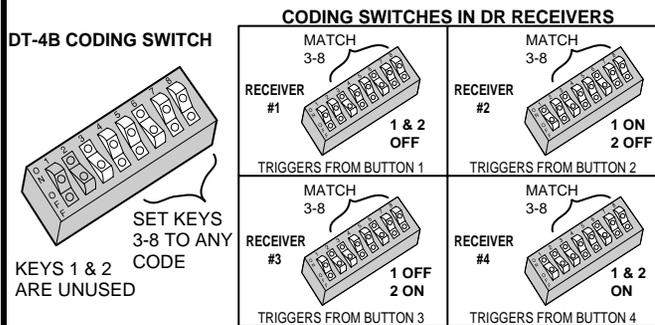
**STEP 2B Coding for two-channel receivers.** Pick any combination of OFF/ON codes and set them on switch keys 3-8 in the transmitter. Match the same code on switch keys 3-8 in each receiver. Set each receiver's switch key 2 to select which transmitter buttons (1 & 2, or 3 & 4) will activate it. **Transmitter switch keys 1 & 2 and receiver switch key 1 are unused and can be in any position.**
