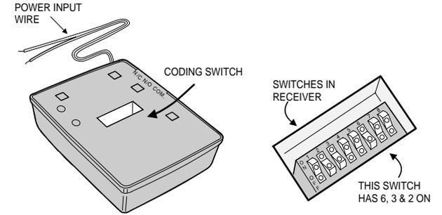
**STEP 1B Transmitter code setting.** Locate the coding switch on the transmitter and set the eight keys identical to those on the receiver. Be sure they are both coded from left to right! Be sure they are identical! If using a two or four-channel transmitter refer to the coding instructions included with the transmitter for proper system coding.
