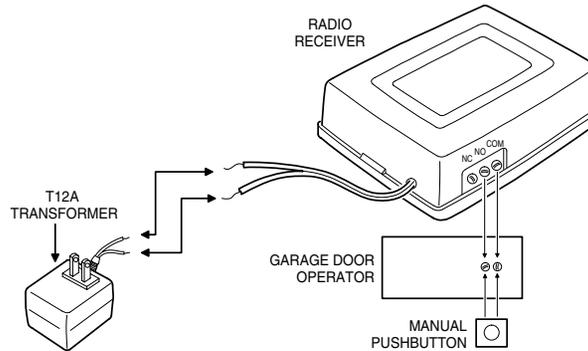
**STEP 2B Connecting receiver (using operator power).** Connect the receiver to the garage door or gate operator as shown in the diagram. Power will be supplied from the operator.
