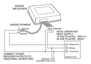
**DESCRIPTION** The Delta-3 DR4V & DR4-12 digital receivers are four-channel wireless radio controls designed for use with automatic garage/gate operators and access control systems. The receivers can be activated by any of the Delta-3 format transmitters. **Receivers must be mounted at least 8 feet apart.** The Delta-3 radio format provides 256 different digital codes. The
