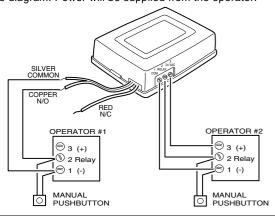
**DESCRIPTION:** The Delta-3 DR-2 digital receiver is a two-channel wireless radio control designed for use with automatic garage/gate operators and access control systems. The receiver can be activated by any of the Delta-3 format transmitters. Receivers must be mounted at least 8 feet apart.
