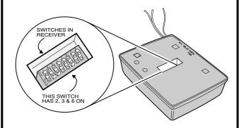
STEP 4A Connecting receiver (using transformer power). A Model 524 transformer can be used to power the receiver when connecting receiver to any operator. Connect as shown, then plug the transformer into a convenient (unswitched) 110 VAC outlet.
