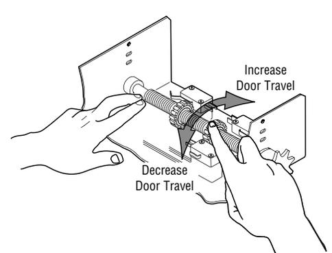
**NOTE:** When retaining plate is released, verify that the retaining plate is fully seated with the notches of the limit nut.
