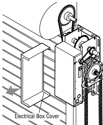
**2** Run power wires to electrical box according to national and local electrical codes.
