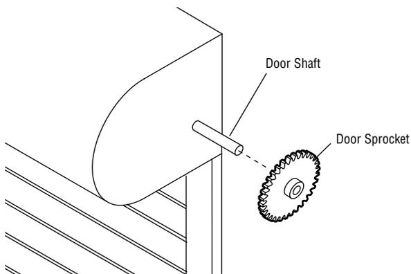
**2** Place operator door sprocket on operator.
