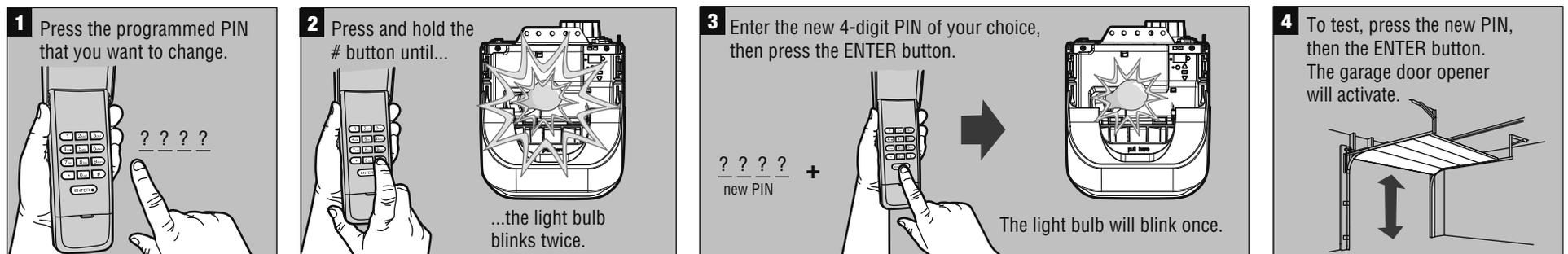
\* For garage door openers that have a green Learn button or an external receiver repeat "Program Initial PIN" to change the existing PIN.
