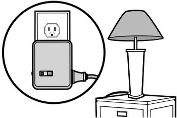
**2** If the lamp is not ON, press and release the Power button on the module to turn the lamp ON.
