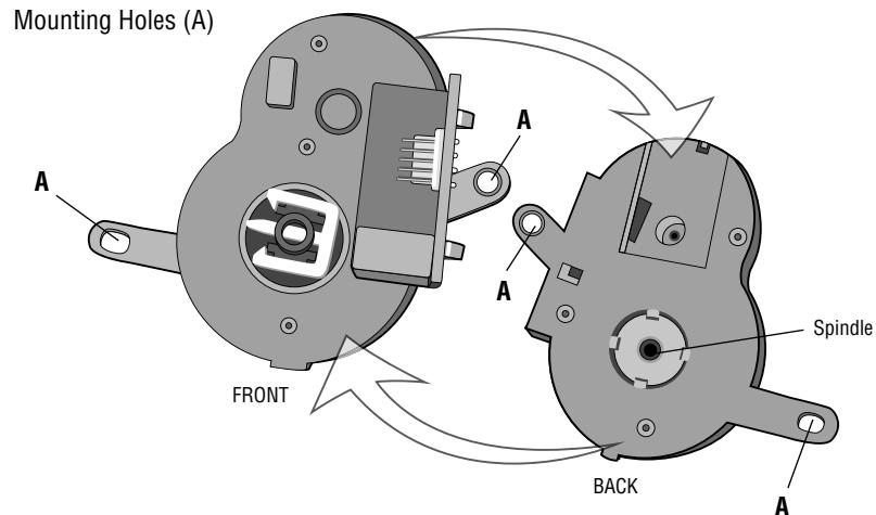
**2.1** Install the new travel module by aligning the spindle to the motor.
