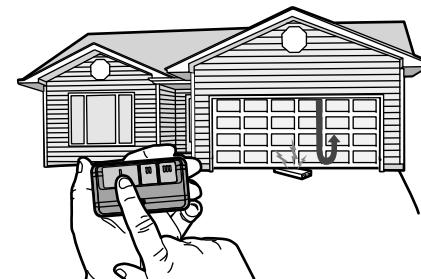
If the door stops and does not reverse on the obstruction, the travel needs to be adjusted (refer to Adjustment Step 1).
