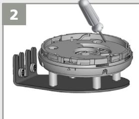
2 Position the bracket and secure using the 4 screws to avoid vibrations.
