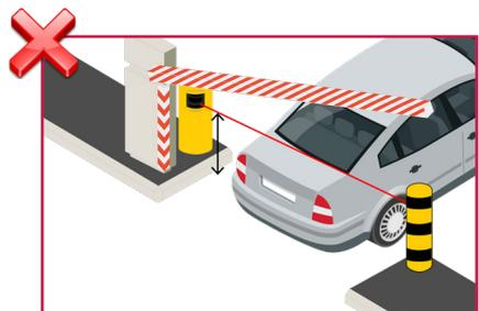
If the 0° reference beam is too low or too high, vehicle contact with the barrier may occur.
