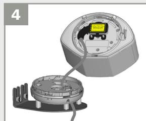
4 Firmly close the protection cover. Do not pinch the cable.
