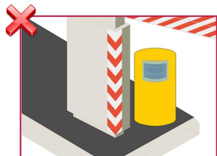
Do not cover the front face of the sensor with glass or plastic.
