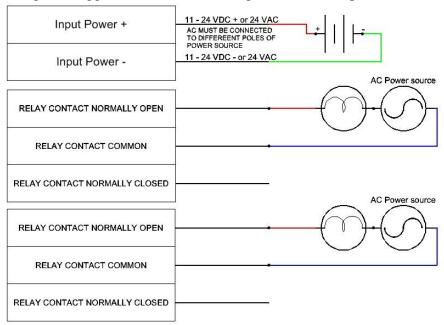
2. To open a gate or door using channel 1 and close with channel 2.
