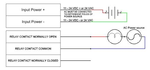
2. To De-energize a Magnetic lock. May be used in and of the operating modes as desired.
