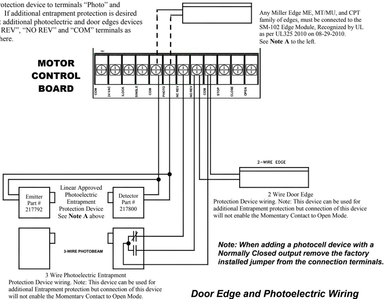
After properly connecting an approved Entrapment Protection Device (see above and Page 3) to the operator, see Pages 15 & 16 for setting of the selector switches. These switches must be properly set and an approved photoelectric device or approved door edge device connected to the operator to obtain B2 Mode of Operation, Momentary Contact to Close.
