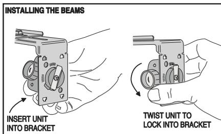
4 Insert the sender and receiver into the bracket holes so the lenses of the units will face each other. Twist the units until the spring clips lock into a detent mark on the brackets. To protect the units from being bumped after installation, it is recommended to mount the sender and receiver inside the brackets as shown.
