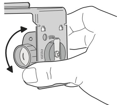
ADJUST THE SENDER AND RECEIVER UNTIL THE RED INDICATOR LIGHTS SOLID
