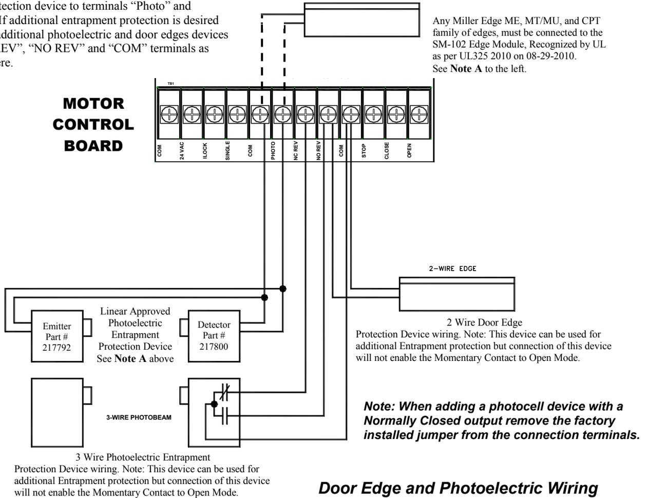
After properly connecting an approved Entrapment Protection Device (see above and Page 3) to the operator, see Page 15 for setting of the selector switches. These switches must be properly set and an approved photoelectric device or approved door edge device connected to the operator to obtain B2 Mode of Operation, Momentary Contact to Close.
