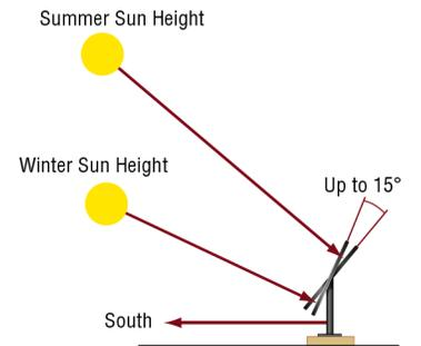
**TIP:** To optimize the system for winter operation the angle can be increased an additional 15° (solar panel(s) sits more vertical).
