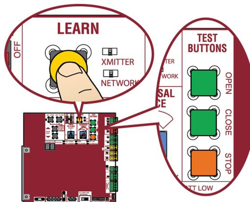
There are 3 different options for programming the remote control depending on how you would like the remote control to function. Choose a programming option:
