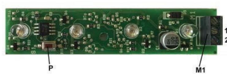
Power 24 V AC/DC supply to pins 1 and 2 on the M1 terminal.
