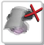
The sensor must be firmly fastened to prevent vibration.
