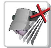
The sensor must not have any object likely to move or vibrate in its sensing field.
