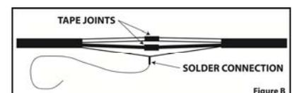
SHIELD drain wire and solder the connection. DO NOT cut off the excess SHIELD drain wire.
