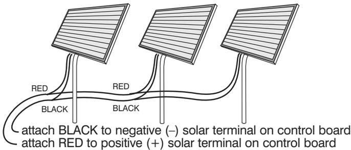
*All connections should be made weatherproof using weatherproof splice kits available at hardware and electrical supply stores.*
