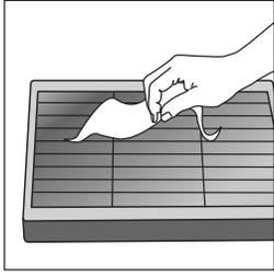
For optimal efficiency, wipe the face of the panel frequently with a soft, damp cloth.
