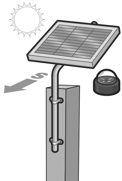
\*If the solar panel must be placed more than 10 ft. from the control box in order to receive direct sunlight, you can use up to 250 ft. of multi-stranded, 16 gauge, direct burial, low-voltage wire [RB509]. **NEVER use telephone wire or solid core wire.**
